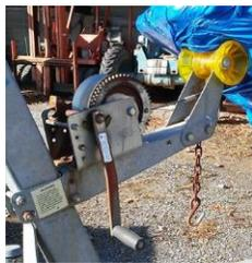
There is a piece of equipment, and its backup, many trailer boaters fail to review as they winterize and store the boat. I refer to the winch and its components. It is down-right embarrassing, and dangerous to have any of the components
