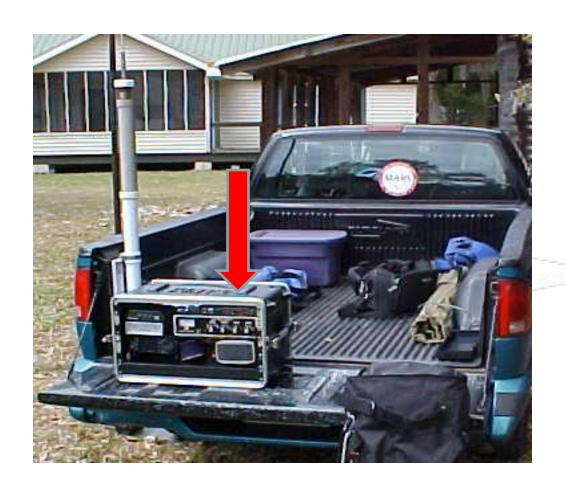
An example of a transportable radio facility is shown on the tailgate of the truck
