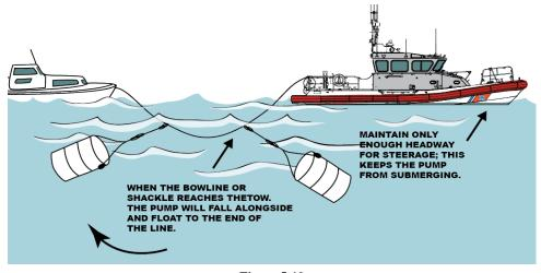
Figure 5-10 Passing a Drop Pump on the Towline
