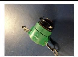
Figure 5-18 **Color-Coded Coupling**
