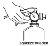
Figure 5-21 Dry Chemical Extinguisher
