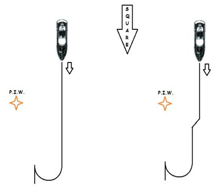
Figure 4-11 Spacing while Traveling Down Swell
