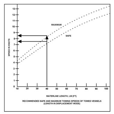
Figure 3-16 Calculated Safe Towing Speeds
