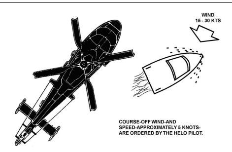
Figure 6-9 Helicopter-Boat Hoist
