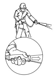
HOLD HORN BY INSULATED HANDLE... SQUEEZE TRIGGER
