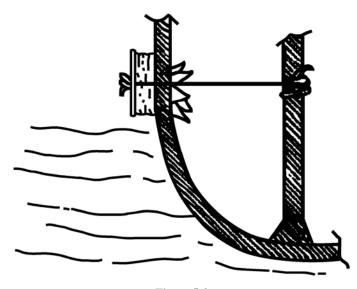
Figure 5-3 **Patching Hole Above Waterline**
