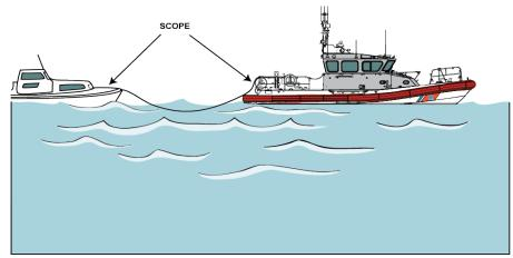
Figure 3-15 **Scope of Towline with Catenary**
